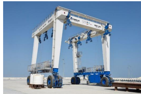
Travel Lift is designed to accommodate vessels of 30.0 meters LOA in length with a weight of 300 tonnes.
